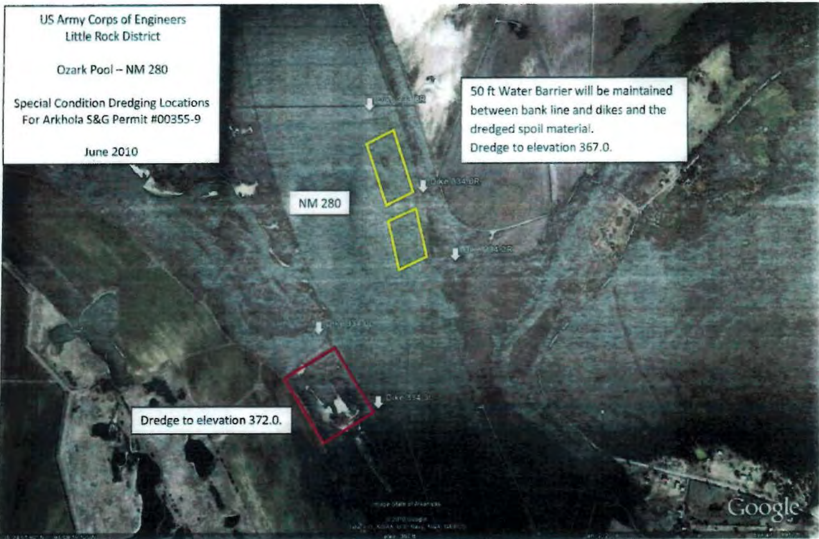
Figure 1. NM 280.4 Left Bank: Dredging of material will be allowed between Dikes 334.0L and 334.3L down to elevation 372.0. NM 279.8-280.2 Right Bank: Dredging of material will be allowed between Dikes 334.2R, 334.0R and 333.8R down to elevation 367.0 to re-establish a water barrier of 50 feet.
